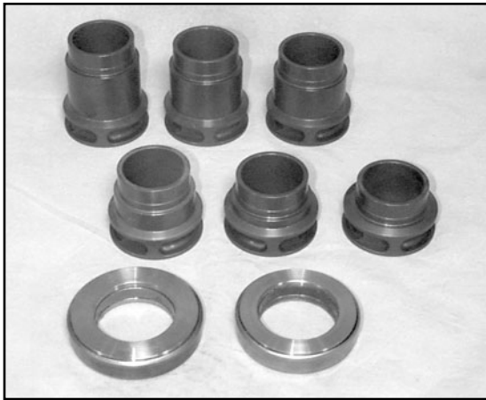
Length measurement is entire length of bearing and collar combined
